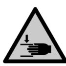
Warning: crushing of hands
